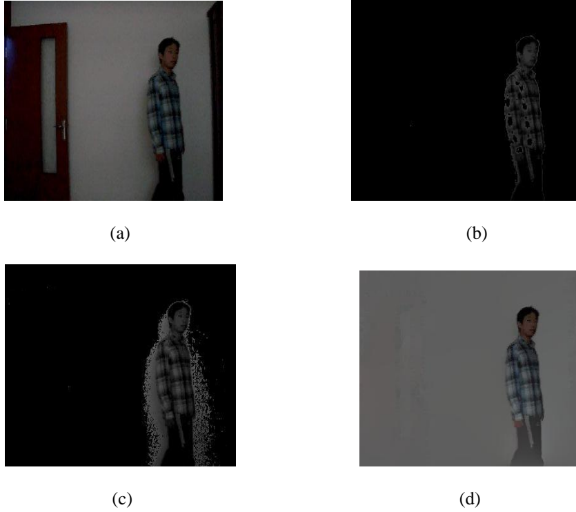
Figure 2: Comparison of Background Subtracted Image Obtained from Three Different Techniques Taken from Man Sequence (a) Input Image (b) Approximate Median (c) Mixture of Gaussian (d) Our Method
