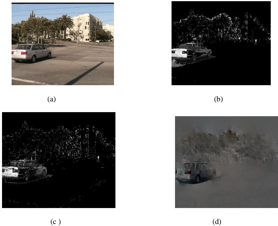
Figure 3: Comparison of Background Subtracted Image Obtained from Three Different Techniques Taken from san_fran_traffic_30sec_QVGA_Cinepak Sequence (a) Input Image (b) Approximate Median (c) Mixture of Gaussian (d) Our Method
